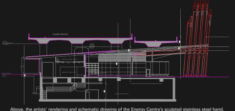
Above, the artists' rendering and schematic drawing of the Energy Centre's sculpted stainless steel hand. The fingernails are LED lighting fixtures that will change colour to reflect the amount of green energy being produced by the system.
