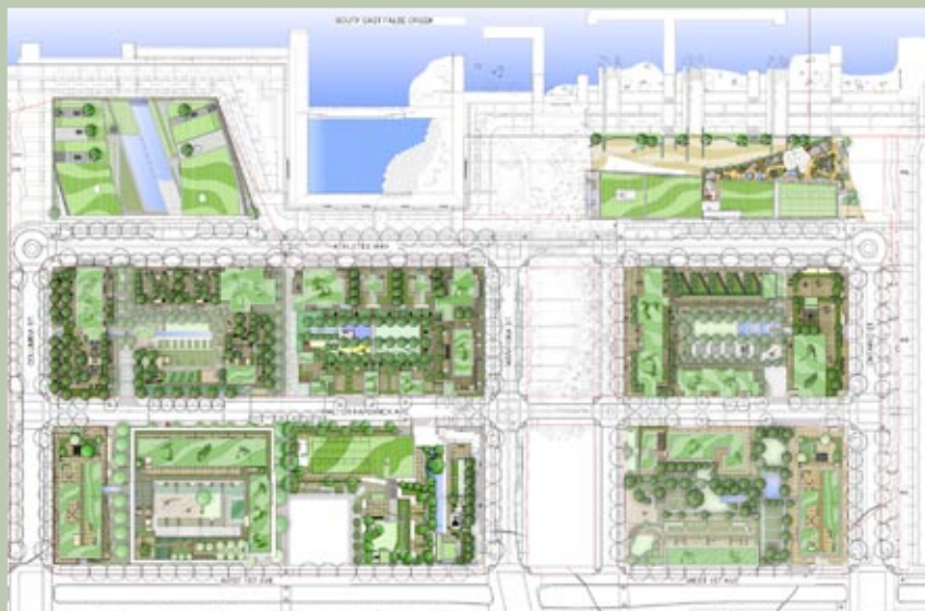
An illustrative plan of the Olympic Village by landscape architects Durante Kreuk highlights the intensity of vegetation on the rooftops throughout the site. Combining intensive and extensive green roofing, fifty percent of the overall area is vegetated.
