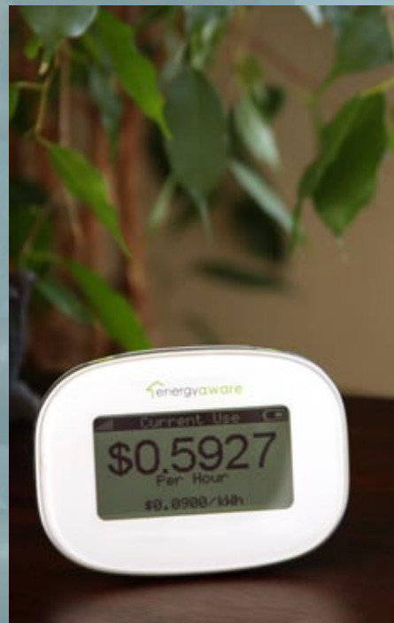
The Energy Aware PowerTab is a display unit that communicates real-time energy and resource use in each suite.
