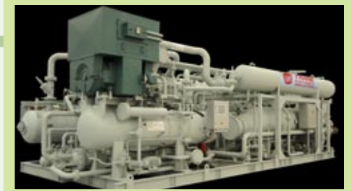
Left: Schematic of the Neighbourhood Energy Utility Above: The NEU sewage heat pump photographed on the factory test stand at Trane's plant.
