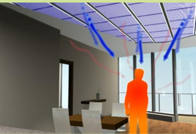
Left and center: Radiant energy transfers heat from a mass with higher temperature to one with lower temperature, in the same way we are warmed by the sun. When the radiant system is switched to cooling, it draws heat from objects – including bodies – that are warmer than the water, giving a cooling effect.
