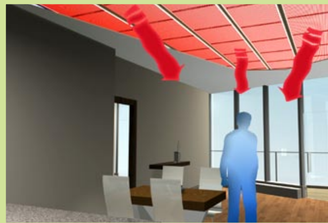
Left and center: Radiant energy transfers heat from a mass with higher temperature to one with lower temperature, in the same way we are warmed by the sun. When the radiant system is switched to cooling, it draws heat from objects – including bodies – that are warmer than the water, giving a cooling effect.
