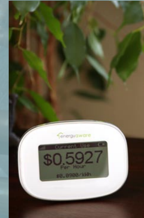
The Energy Aware PowerTab is a display unit that communicates real-time energy and resource use in each suite.
