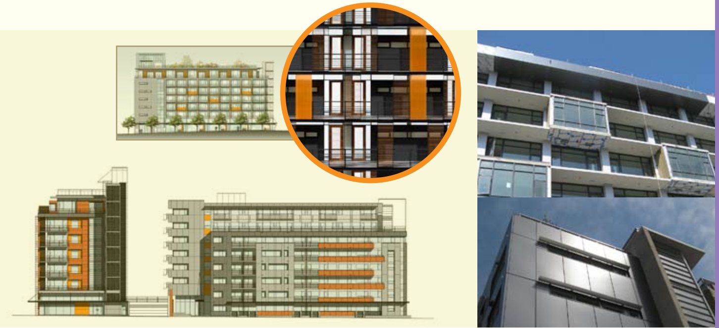
Elevation drawings show Parcel 5’s buildings as seen from the north on Walter Hardwick Avenue (bottom) and from the east on Manitoba Street. Inset detail of the scale model shows the colour palette of deep orange and dark greys. Construction photos taken August 2009.
