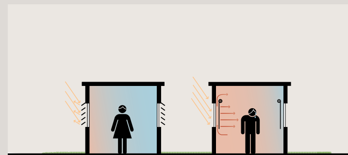
EXTERIOR VS INTERIOR SHADING The choice of shading devices can greatly affect a building’s cooling capacity. Shades on the exterior of a building block the sun before it meets the building envelope. Interior shades allow the sun’s energy to penetrate the window, heating up the building’s interior.
