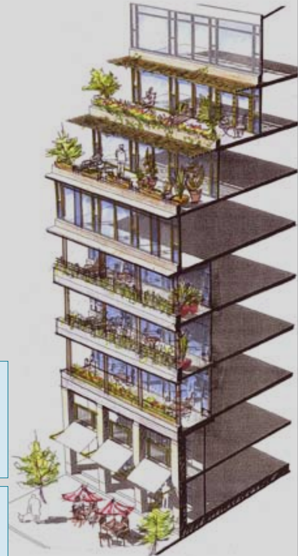
Shading is a key passive design strategy that can be achieved by incorporating balcony overhangs, plants and trees, and active blind systems.
