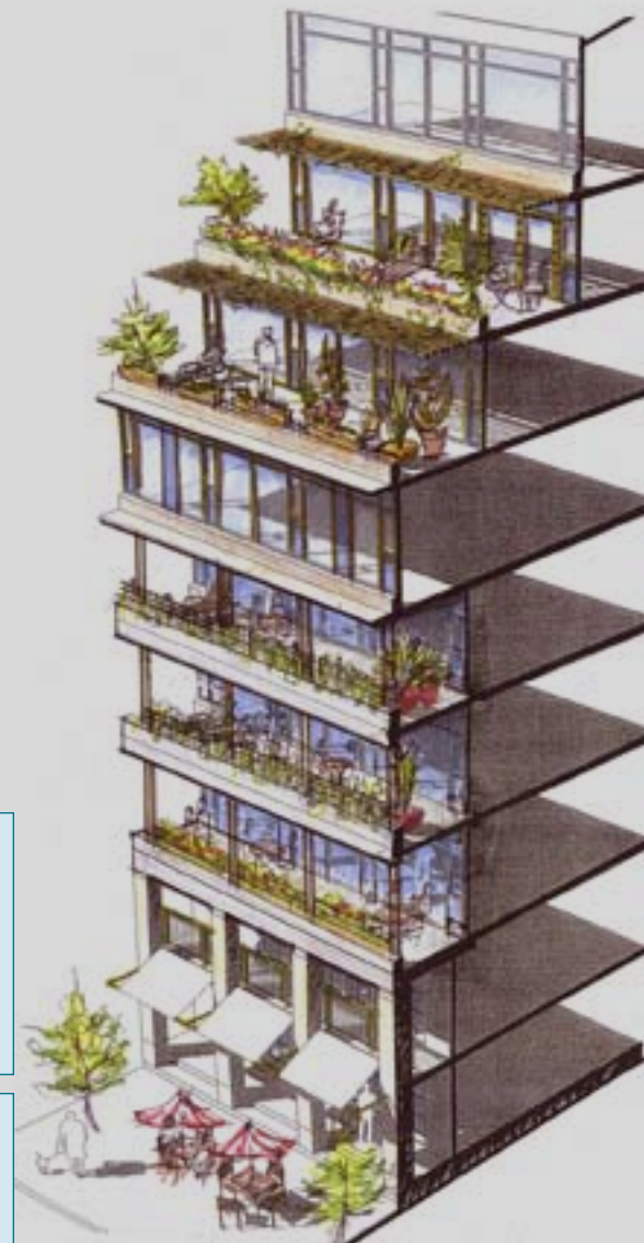
Shading is a key passive design strategy that can be achieved by incorporating balcony overhangs, plants and trees, and active blind systems.
